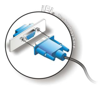
Figure 3-31: VGA Connector
