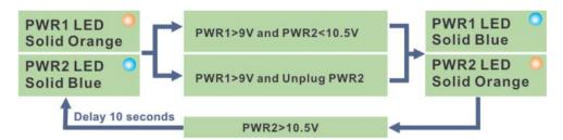
Figure 3-41: ACC Off: Switch Between PWR1 and PWR2
