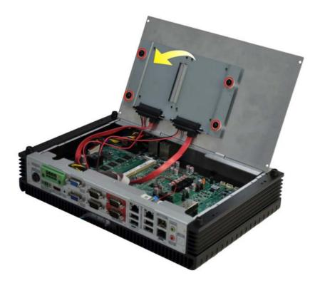
Figure 3-2: HDD Bracket Retention Screws
