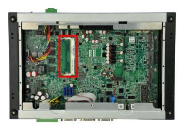
Figure 3-9: SO-DIMM Socket
