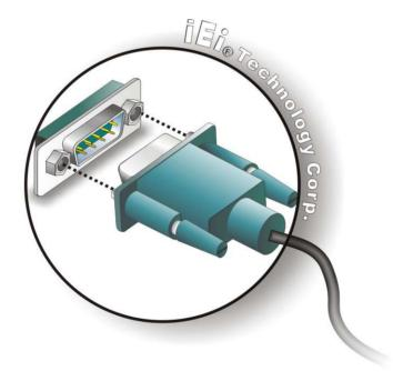
Figure 3-28: Serial Device Connector
