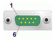
Figure 3-16: DIO Connector Pinout Location
