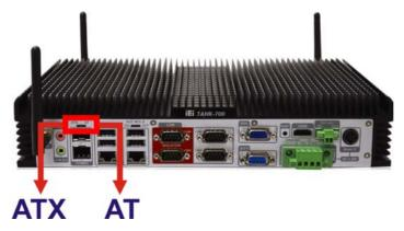
Figure 3-13: AT/ATX Power Mode Switch
