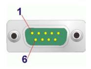
Figure 3-24: DB-9 Connector Pinout Location
