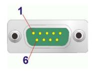
Figure 3-29: Serial Port Pinout Location
