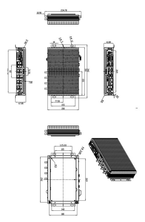
Figure 1-5: Physical Dimensions (millimeters)
