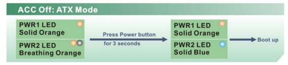
Figure 3-40: ACC Off: ATX Mode
