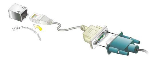
Figure 3-22: RJ-45 RS-232 Serial Device Connection
