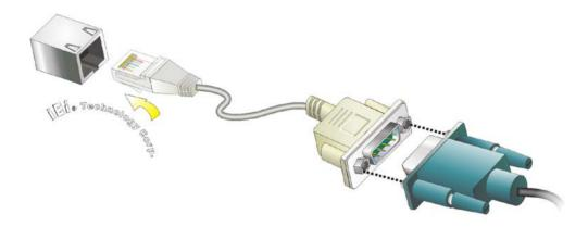
Figure 3-25: RJ-45 RS-422/485 Serial Device Connection
