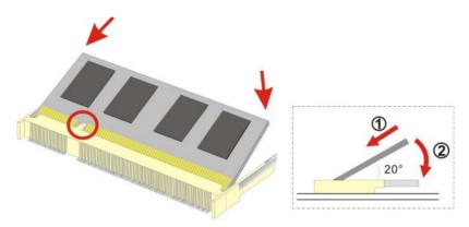
Figure 3-10: SO-DIMM Installation
