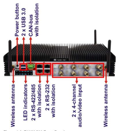
Figure 1-2: TANK-700 Front Panel
