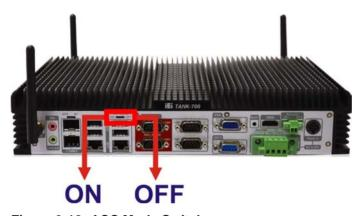
Figure 3-12: ACC Mode Switch
