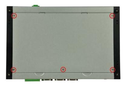
Figure 3-1: Bottom Panel Retention Screws
