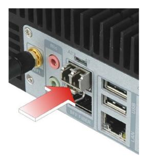
Figure 3-8: SFP Module Installation
