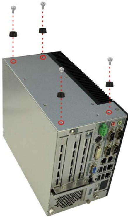
Figure 3-10: Foot Pad Installation
