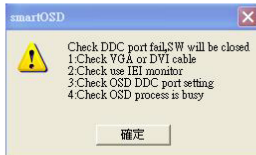
Figure C-13: DCC Port Failure
