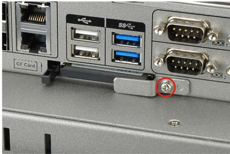
Figure 3-9: Replacing the CompactFlash® Cover Plate
