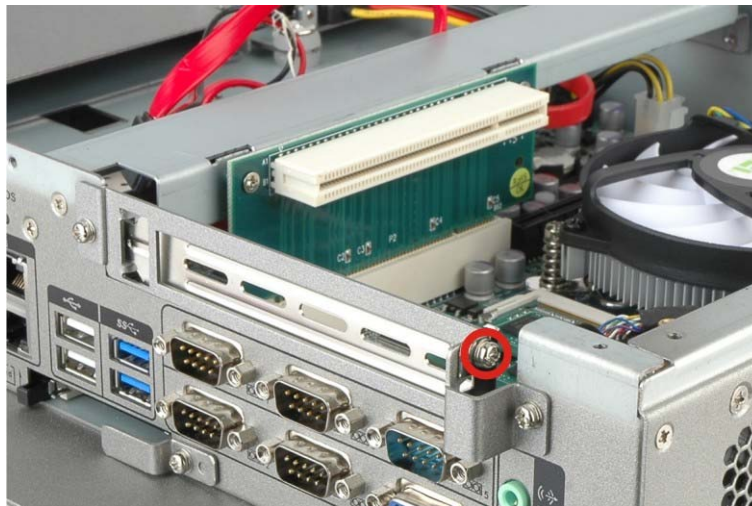
Figure 3-16: Expansion Slot Retention Screw
