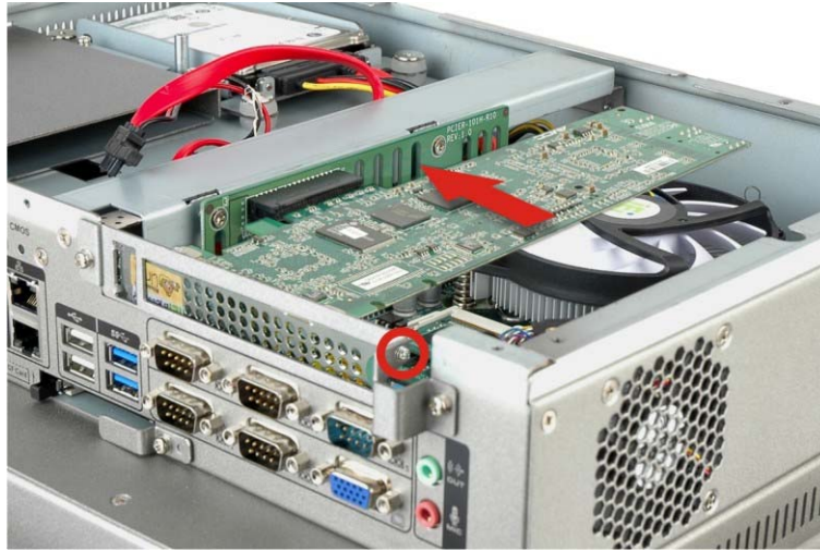
Figure 3-20: Installing the PCIe Card
