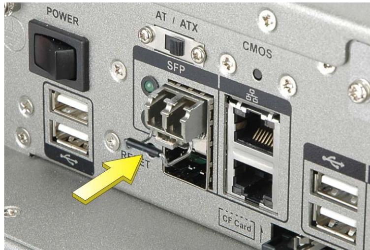
Figure 3-32: SFP Fiber Module Installation
