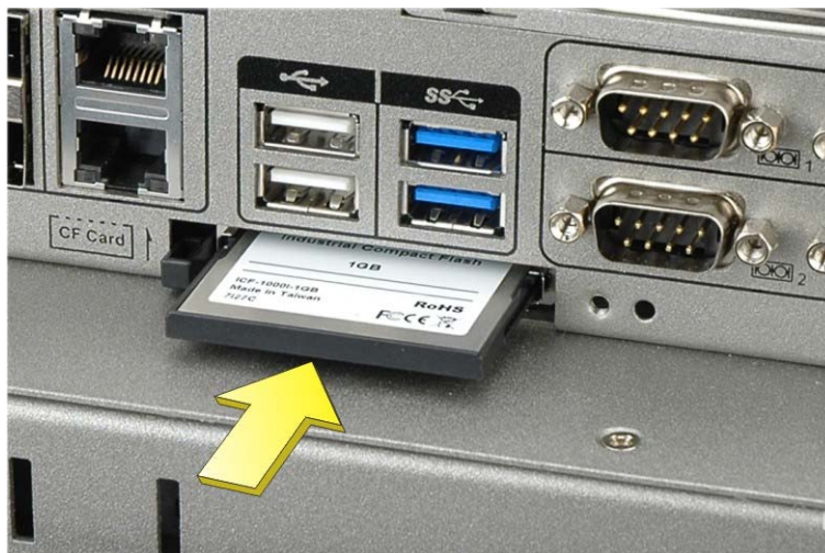
Figure 3-8: Installing the CompactFlash® Card
