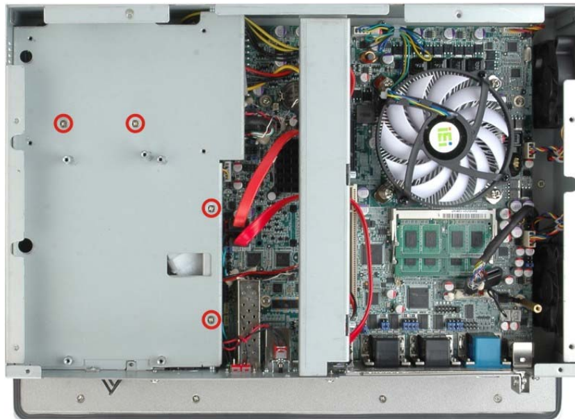
Figure 4-6: PPC-5150A-H61 Internal Elevated Platform Screws
