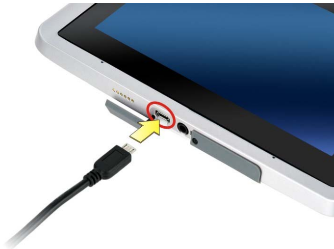
Figure 3-2: Connecting the Micro USB Cable to the ICELOG-07
