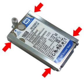
Figure 4-5: Securing the HDD
