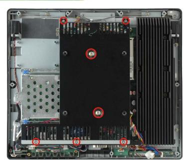
Figure 5-2: Internal Cover Retention Screws
