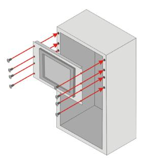
Figure 4-13: Install into a Rack/Cabinet
