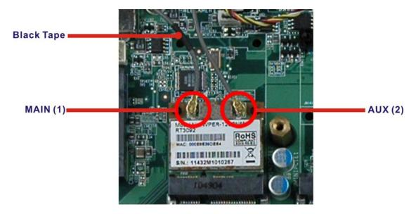
Figure 5-7: Attaching the Antennas
