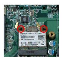
Figure 5-5: Releasing the WLAN Card
