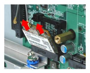
Figure 5-6: Removing the WLAN card
