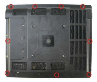
Figure 5-1: Back Cover Retention Screws
