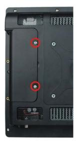
Figure 4-1: HDD Cover Retention Screws
