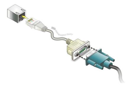
Figure 4-22: RJ-45 Serial Port Connector
