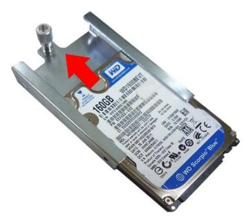
Figure 4-4: Inserting the HDD
