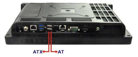
Figure 4-6: AT/ATX Switch Location
