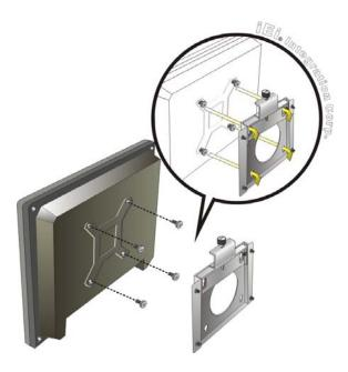
Figure 4-17: Chassis Support Screws
