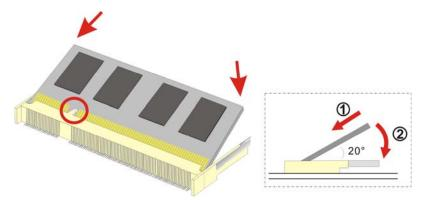
Figure 5-3: DDR SO-DIMM Module Installation
