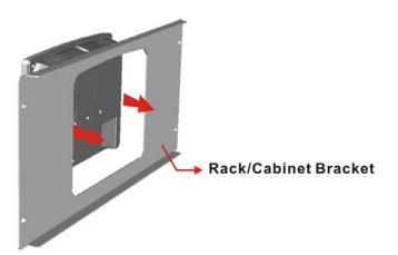
Figure 4-11: The Rack/Cabinet Bracket
