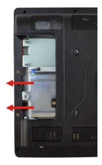
Figure 4-3: Removing the HDD Bracket
