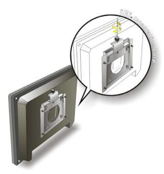
Figure 4-18: Secure the Panel PC
