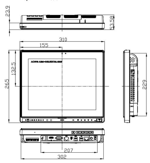
Figure 2-1: AFL2-12A-HM65 Dimensions (mm)
