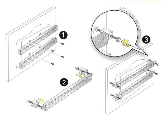
Figure 4-12: Rack Bracket Mounting
