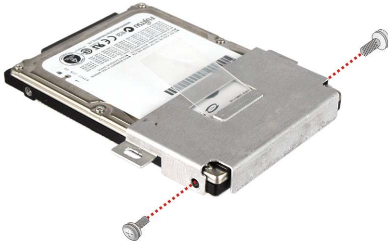
Figure 2-3: HDD Bracket Retention Screws
