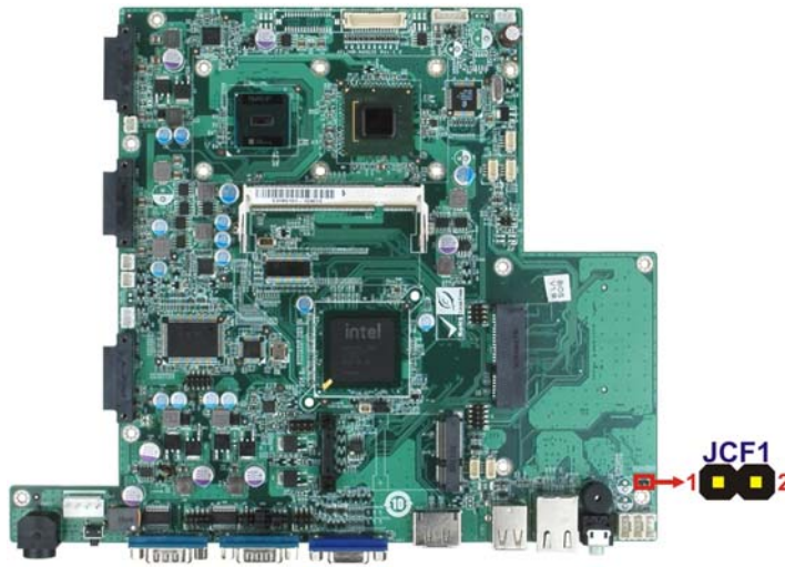
Figure 2-10: CF Card Setup Jumper Location
