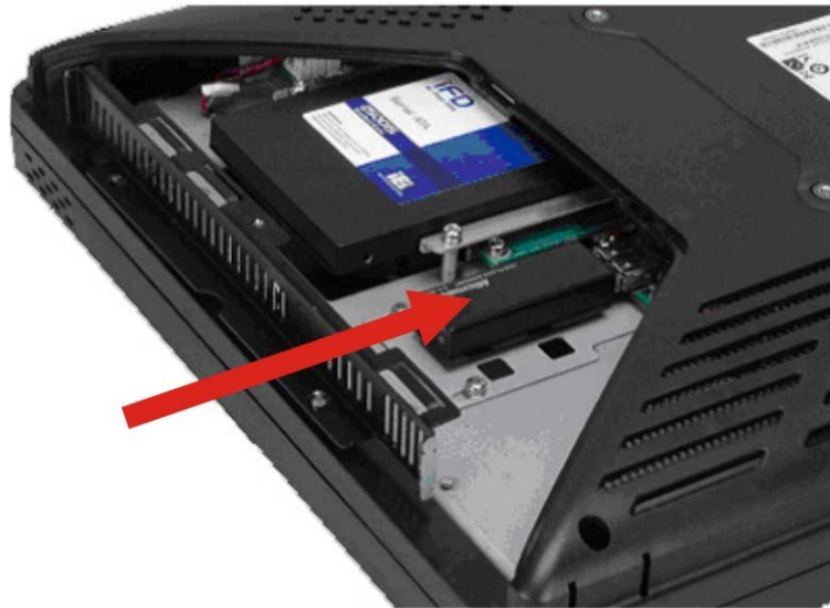
Figure 2-7: USB Dongle Installation
