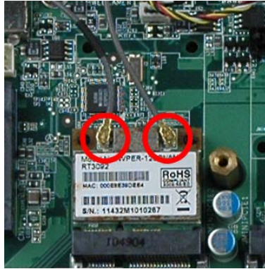
Figure 7-5: Removing the Antennas
