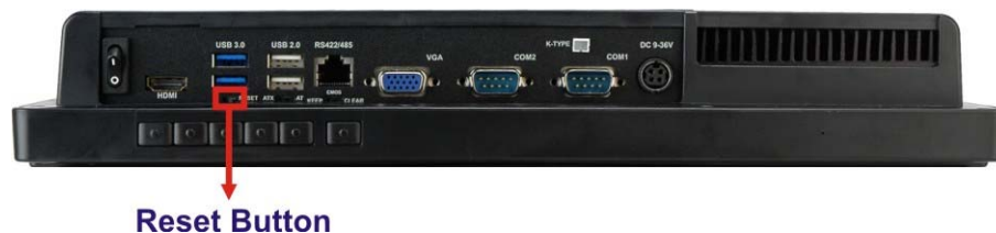
Figure 3-13: Reset Button Location
