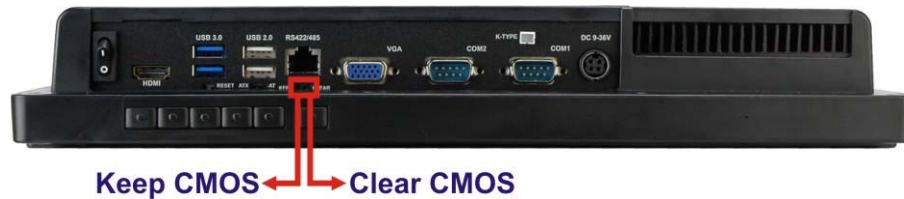
Figure 3-12: Clear CMOS Switch Location
