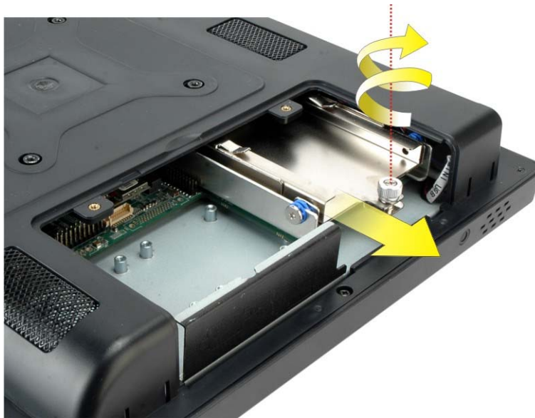
Figure 3-2: HDD Bracket Removal
