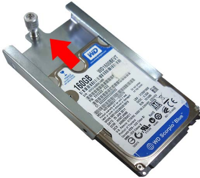
Figure 3-3: Inserting the HDD
