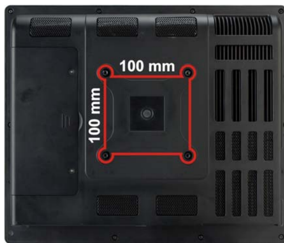
Figure 3-17: Arm Mounting Retention Screw Holes
