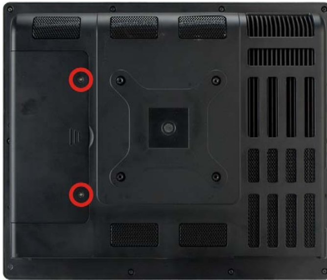
Figure 3-1: HDD Cover Retention Screws
