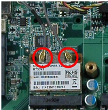
Figure 7-5: Removing the Antennas
