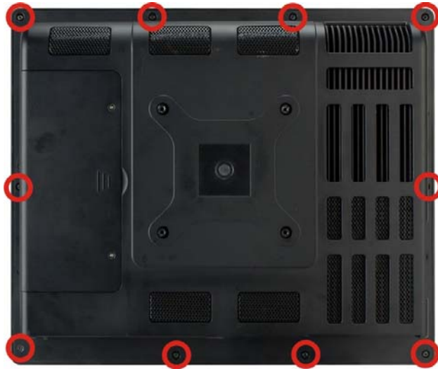
Figure 3-7: Back Cover Retention Screws
