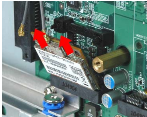
Figure 7-7: Removing the WLAN card
