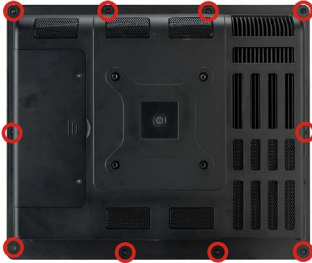
Figure 7-1: Back Cover Retention Screws
