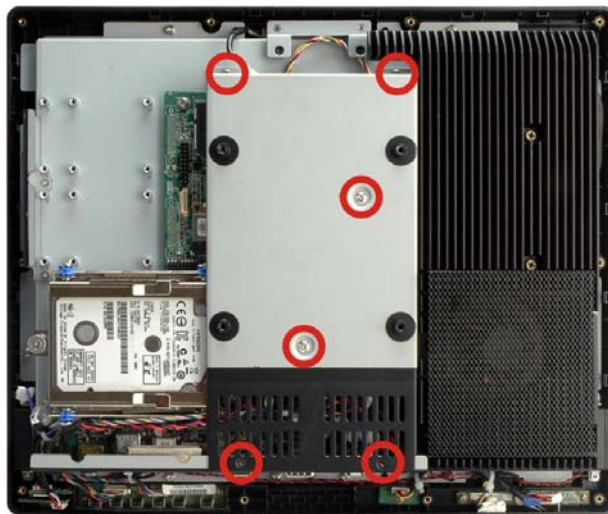
Figure 3-8: Internal Cover Retention Screws
