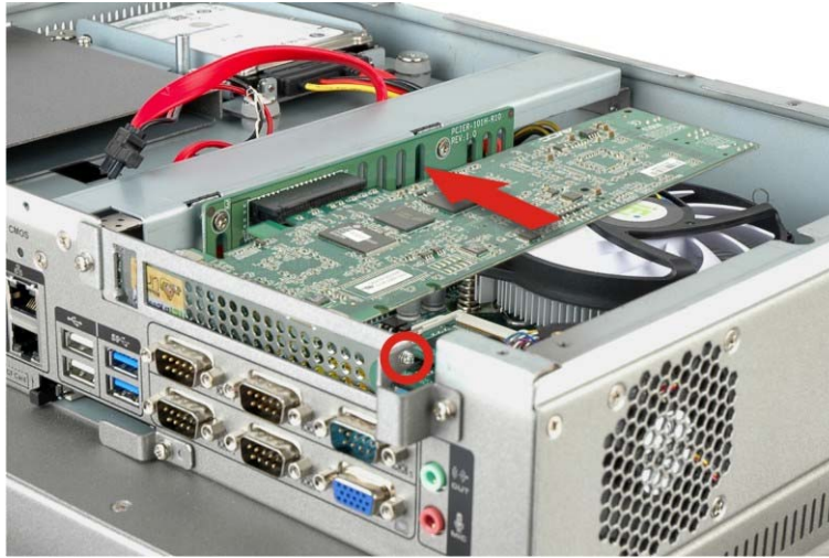
Figure 3-20: Installing the PCIe Card
