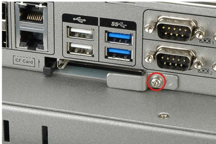
Figure 3-7: CompactFlash® Cover Plate
