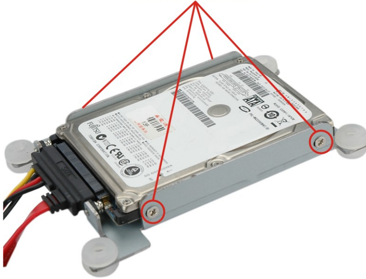
Figure 3-5: HDD Retention Screws
