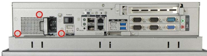
Figure 4-9: PSU Bottom Panel Screws
