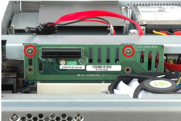
Figure 3-18: Installing the PCIe Riser Card
