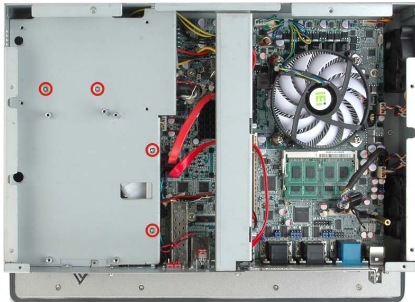
Figure 4-6: WIDS-515A-H61 Internal Elevated Platform Screws
