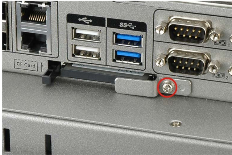
Figure 3-9: Replacing the CompactFlash® Cover Plate
