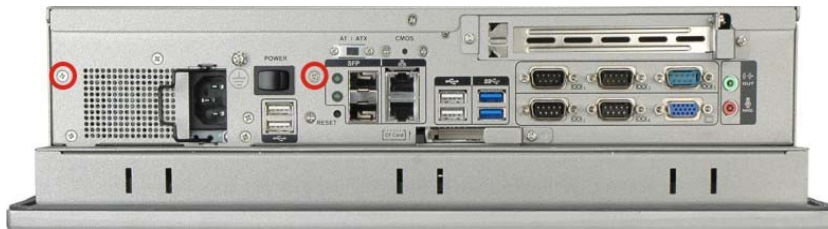
Figure 4-5: WIDS-515A-H61 Bottom Panel Elevated Platform Screws
