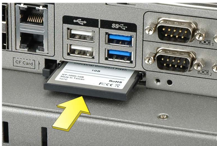
Figure 3-8: Installing the CompactFlash® Card
