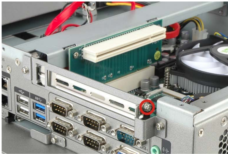
Figure 3-16: Expansion Slot Retention Screw
