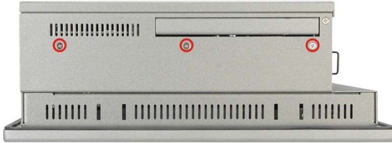
Figure 4-4: WIDS-515A-H61 Side Panel Elevated Platform Screws
