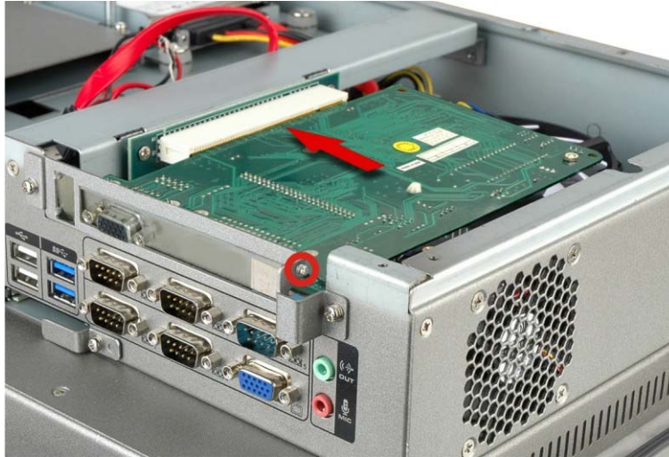
Figure 3-17: Installing the PCI Card
