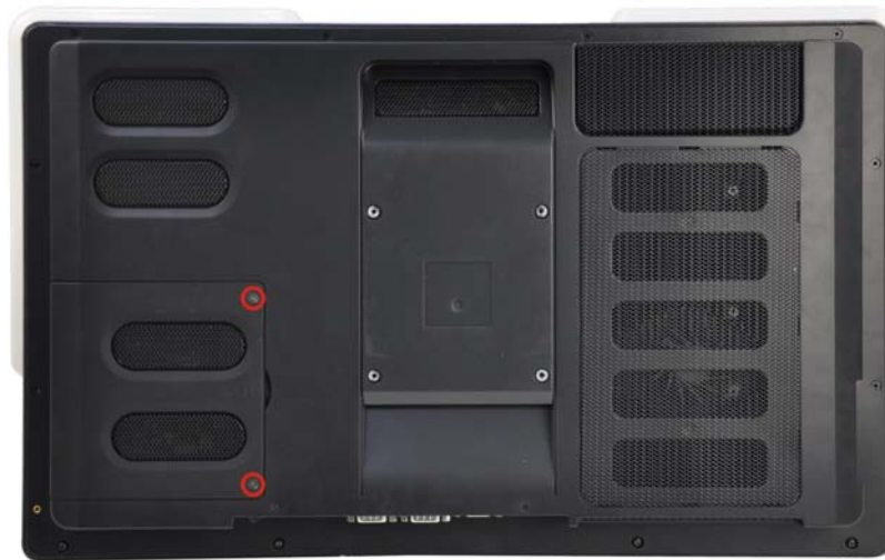
Figure 4-1: HDD Cover Retention Screws
