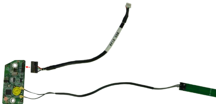
Figure 4-7: Connect the RFID USB cable
