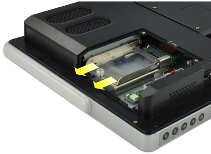
Figure 4-3: Removing the HDD Bracket
