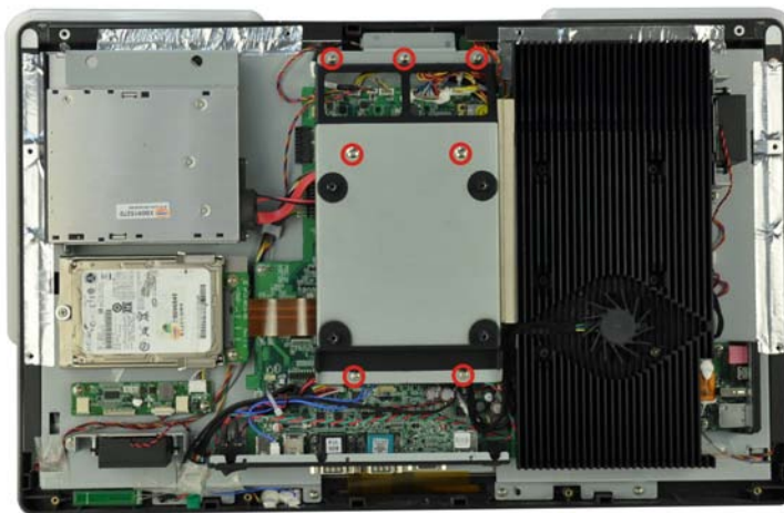
Figure 6-2: Internal Cover Retention Screws
