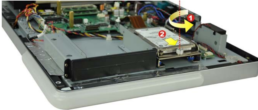
Figure 4-10: Remove the HDD Bracket
