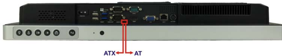
Figure 4-13: AT/ATX Switch Location
