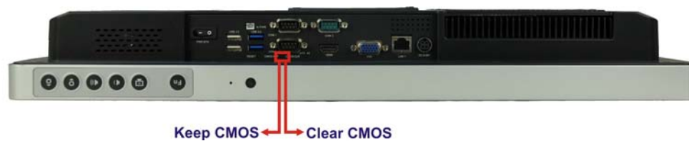
Figure 4-14: Clear CMOS Switch Location
