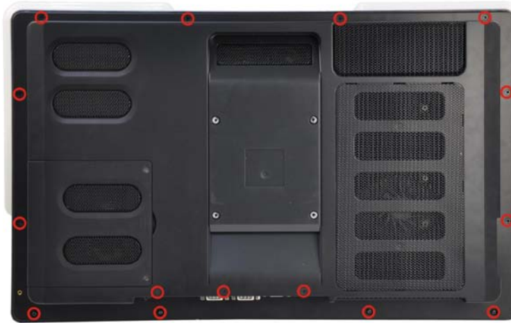
Figure 6-1: Back Cover Retention Screws
