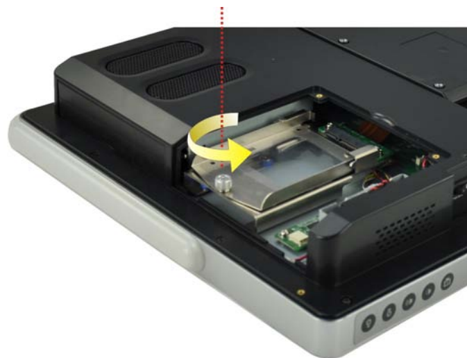
Figure 4-2: HDD Bracket Screw
