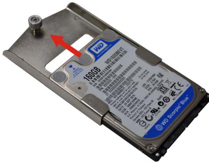
Figure 4-4: Inserting the HDD
