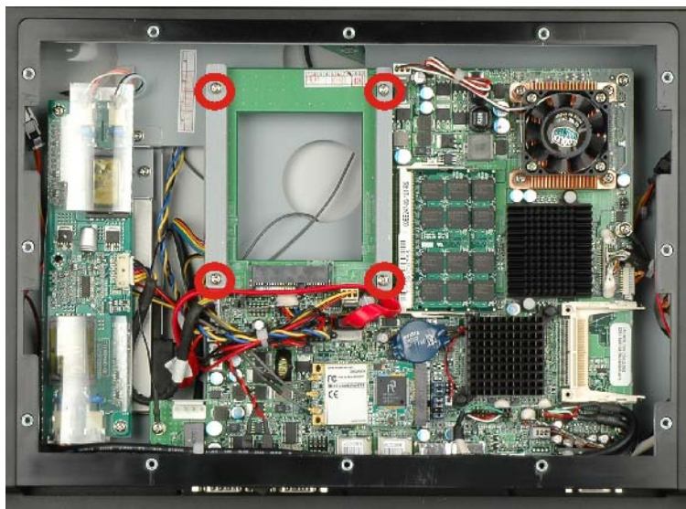
Figure 2-2: HDD Bracket Retention Screws
