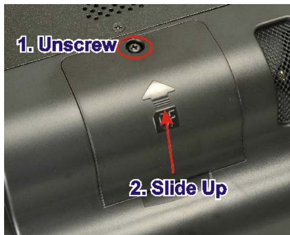
Figure 2–5: Remove CompactFlash® Cover
