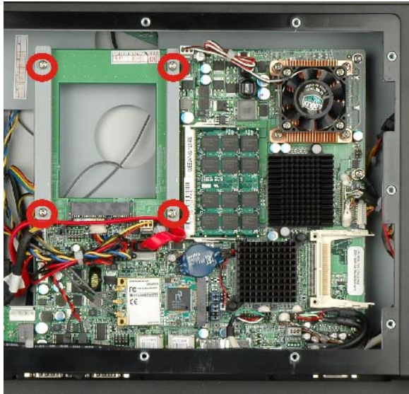
Figure 2-2: HDD Bracket Retention Screws
