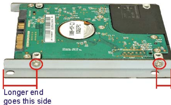
Figure 2-3: HDD Retention Screws
