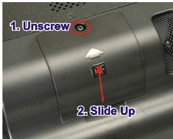
Figure 2-5: Remove CompactFlash® Cover
