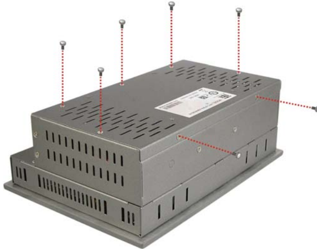
Figure 3-1: PPC-3708A-N26 Back Cover Retention Screws
