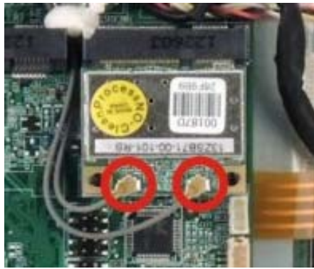
Figure 4-3: Removing the Antennas
