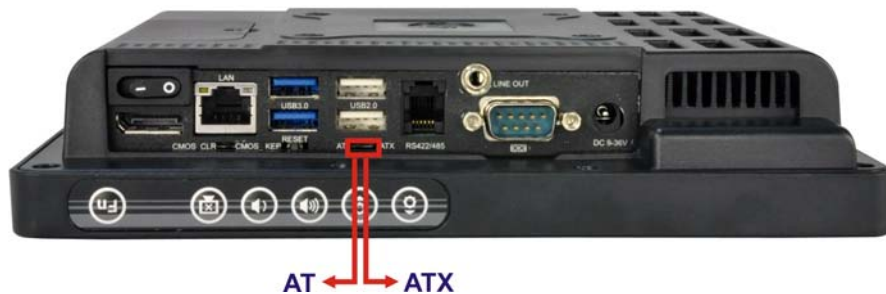
Figure 4-6: AT/ATX Switch Location
