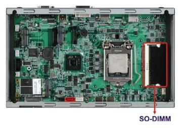
Figure 5-4: SO-DIMM Removal
