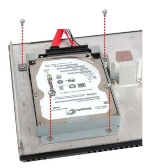
Figure 3-7: Installing the HDD
