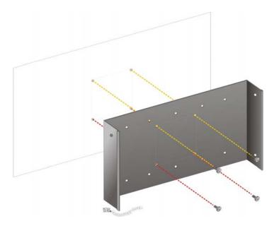
Figure 3-8: Installing the Mounting Bracket
