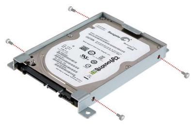
Figure 3-5: Inserting the HDD
