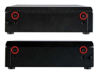
Figure 3-3: Top Cover Retention Screws
