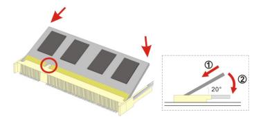
Figure 5-5: SO-DIMM Installation
