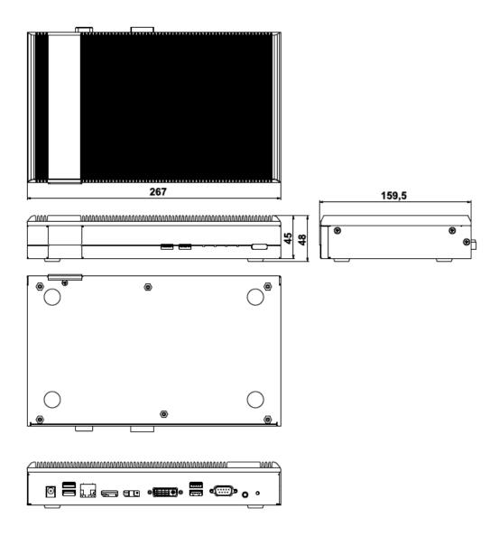
Figure 1-5: IDS-H61 Dimensions (mm)
