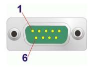
Figure 3-14: Serial Port Pinouts
