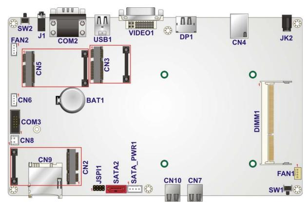
Figure 6-1: Main Board Layout Diagram (Front Side)
