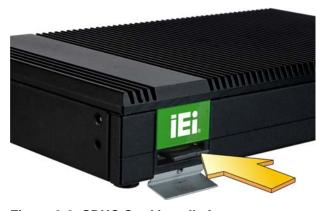
Figure 3-2: SDHC Card Installation
