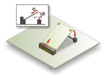
Figure 5-3: mSATA Module Installation
