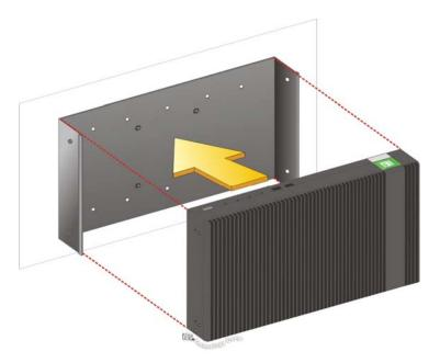
Figure 3-9: Pace the System onto the Mounting Bracket
