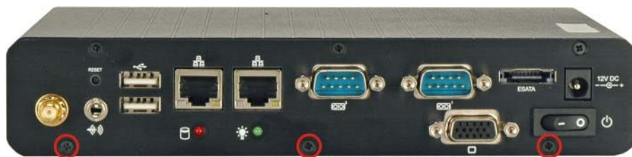
Figure 4-1: Bottom Cover Retention Screws (Front Panel)
