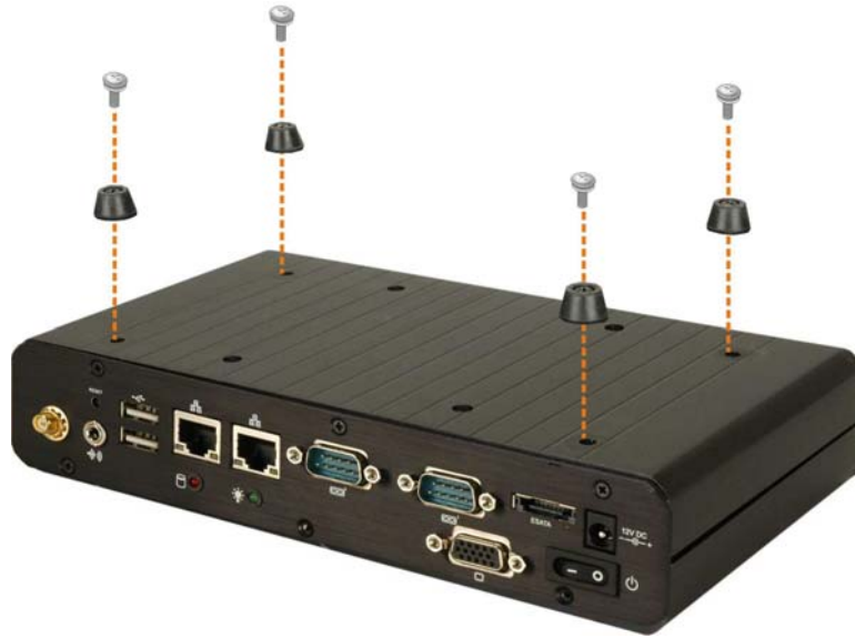
Figure 4-4: Foot Pads Installation
