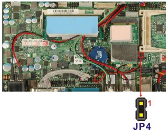
Figure 3-2: AT Power Select Jumper Location
