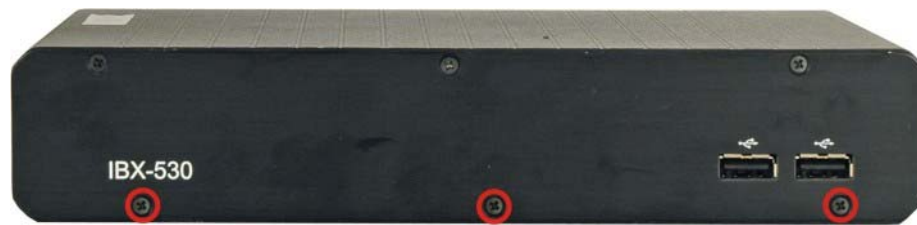
Figure 4-2: Bottom Cover Retention Screws (Rear Panel)
