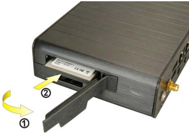
Figure 4-3: CF Card Installation
