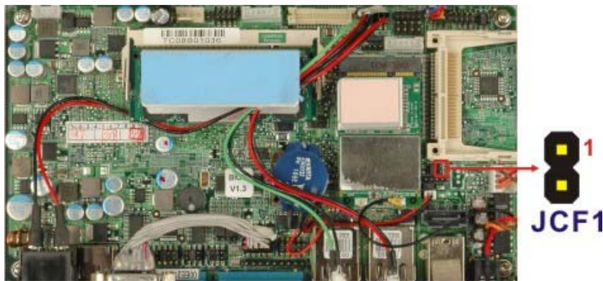
Figure 3-3: CF Card Setup Jumper Location
