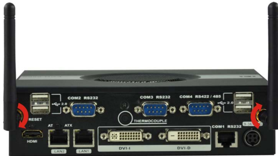
Figure 3-14: Wi-Fi Antenna Installation
