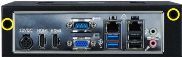
Figure 6: Knockout Holes for Wireless Antenna
