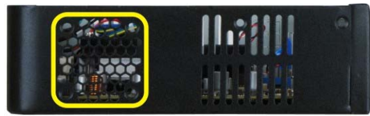
Figure 13: Vents for System Fan
