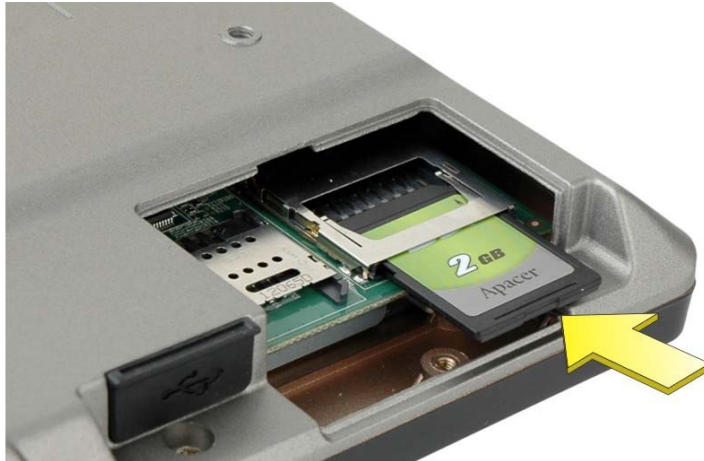
Figure 3-2: Install the SD Card
