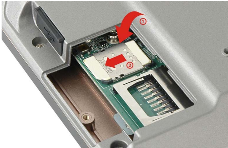
Figure 3-7: Lock the SIM Card Slot Cover
