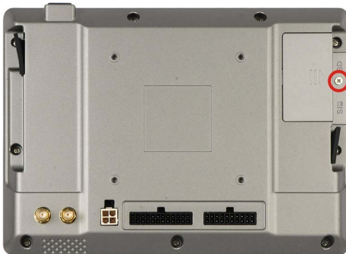
Figure 3-3: SIM Card Slot Access Panel Retention Screw
