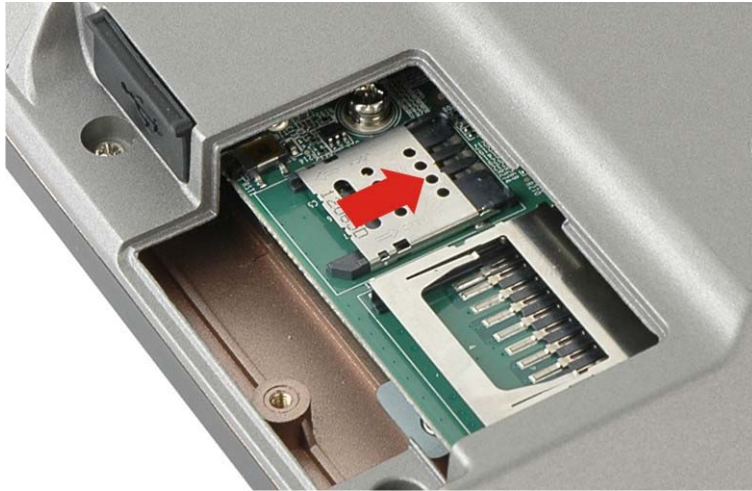
Figure 3-4: Unlock the SIM Card Slot Cover
