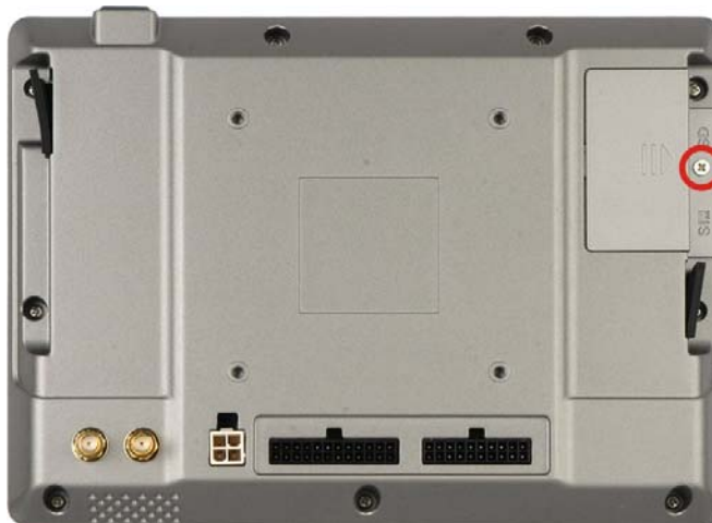
Figure 3-1: SD Card Slot Access Panel Retention Screw
