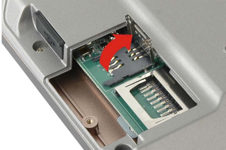
Figure 3-5: Open the SIM Card Slot Cover
