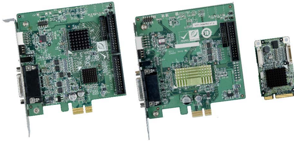
Figure 1-1: IVCE-C608/IVCE-C604/IVCME-C604 Capture Cards
