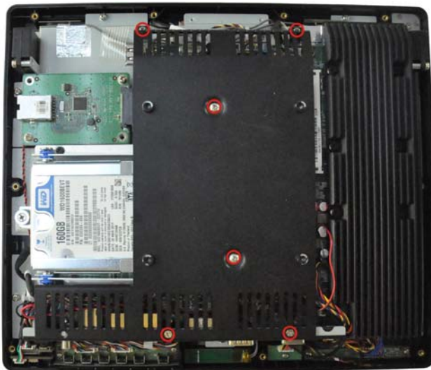
Figure 5-2: Internal Cover Retention Screws
