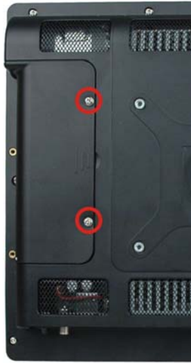
Figure 4-1: HDD Cover Retention Screws
