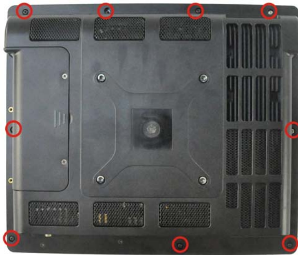
Figure 5-1: Back Cover Retention Screws
