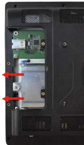
Figure 4-3: Removing the HDD Bracket
