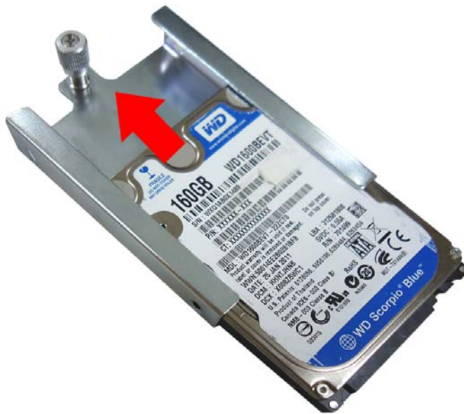
Figure 4-4: Inserting the HDD
