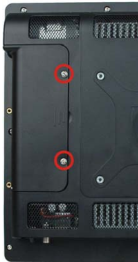
Figure 4-6: HDD Cover Retention Screws
