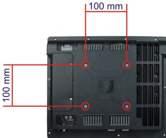
Figure 4-13: Mounting screw location
