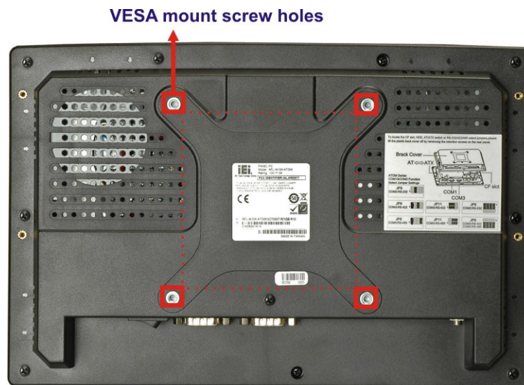
Figure 2-19: AFL-W10A-N270 Arm Mounting Retention Screw Holes
