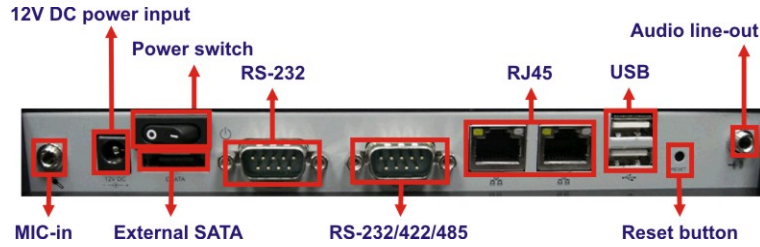
Figure 1-4: AFL-W10A-N270 I/O Interface Connector Panel
