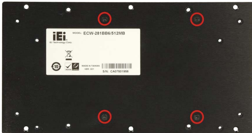
Figure 4-3:HDD Bracket Retention Screws
