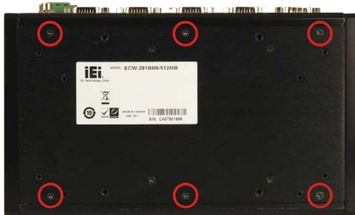
Figure 4-1: Bottom Surface Retention Screws
