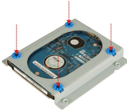
Figure 4-4: HDD Retention Screws
