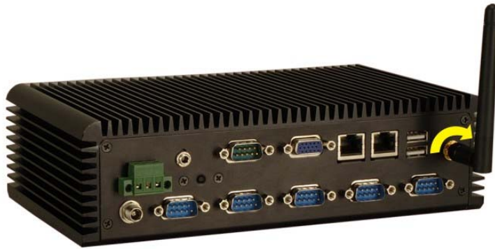
Figure 4-13: Wireless Antenna Installation
