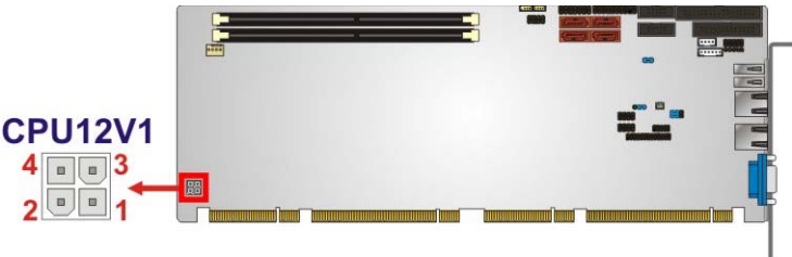
Figure 3-4: ATX Power Connector Pinout Location
