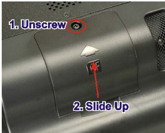
Figure 2-4: Remove CompactFlash® Cover
