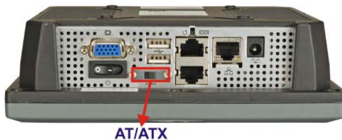
Figure 3-3: AT/ATX Switch Location
