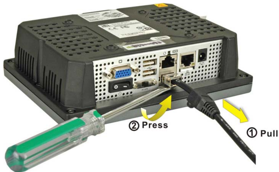
Figure 3-12: Serial Cable Removal
