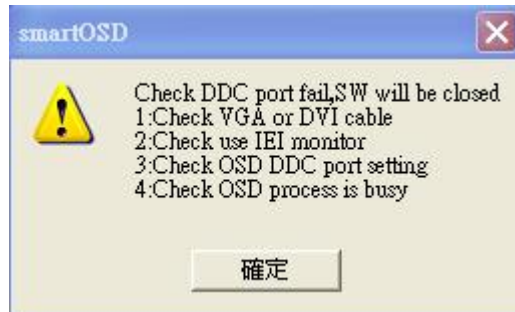
Figure C-13: DCC Port Failure
