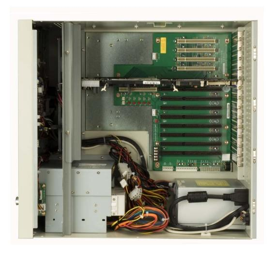
Figure 4-13: Install the CPU Card
