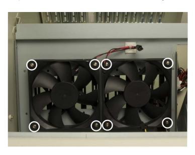
Figure 5-8: Cooling Fan Screws
