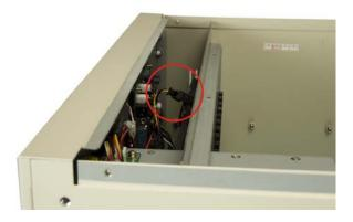
Figure 5-4: Disconnect the Cooling Fan
