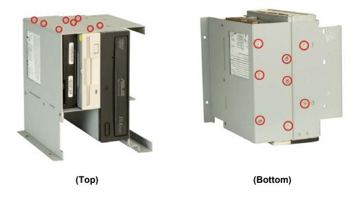
Figure 4-8: 5.25" Disk Drive Retention Screws
