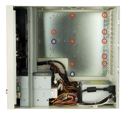
Figure 4-10: Install Copper Pillars and White Spacers
