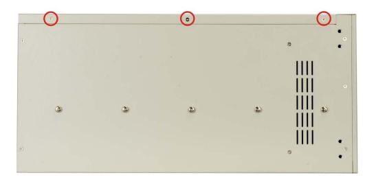
Figure 4-1: Top Cover Retention Screws
