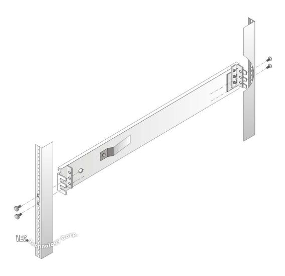
Figure 4-19: Rack Slide Bracket Installation
