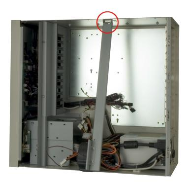
Figure 4-5: Unhook the CPU Card Clamp
