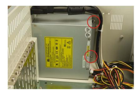
Figure 5-2: PSU Internal Retention Screws
