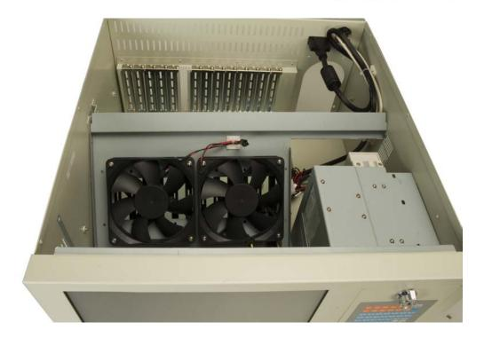
Figure 5-7: Push the Fan Bracket Toward the Rear Panel
