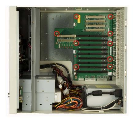
Figure 4-11: Backplane Retention Screws
