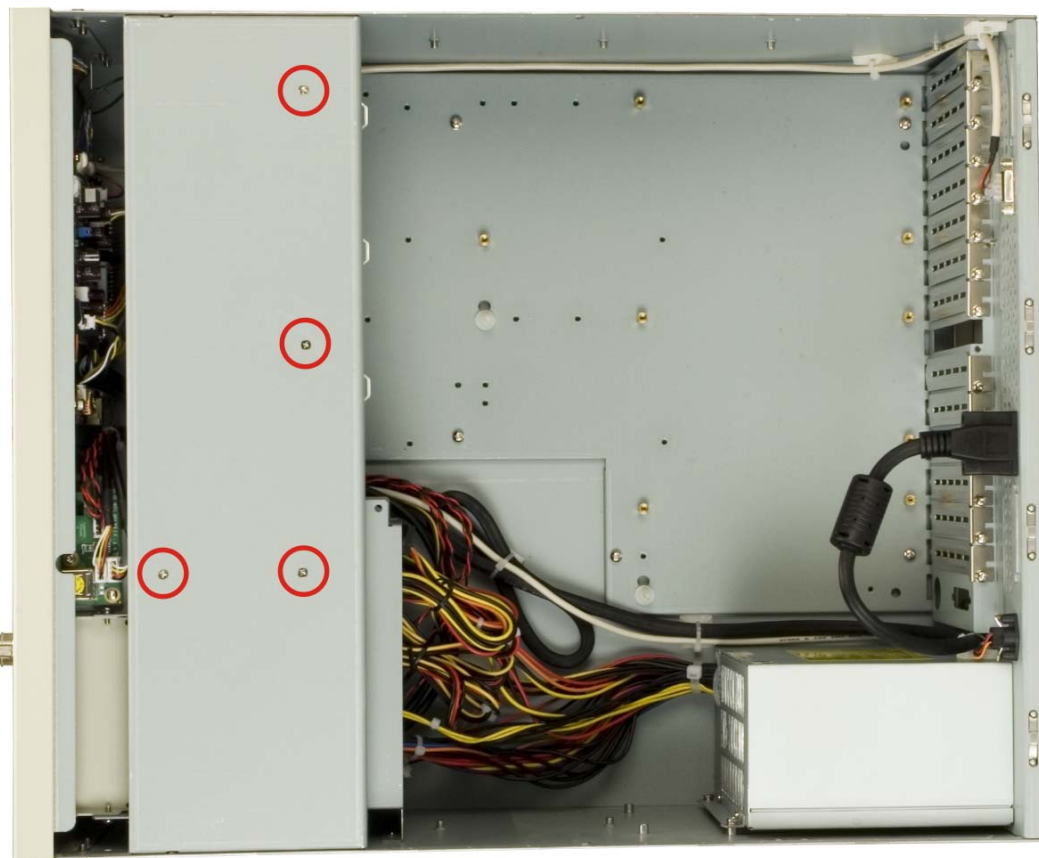
Figure 4-5: Dual CPU Card Clamp and Drive Bay Stabilizer Bracket to Fan Bracket Retention Screws
