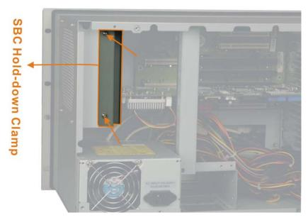
Figure 2-8: Installing the SBC Hold-down Clamp
