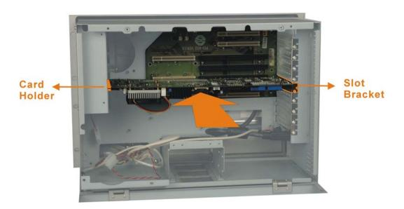
Figure 2-5: CPU Card Installation
