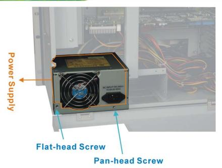
Figure 2-13: Power Supply Installation
