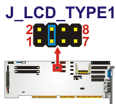
Figure 4-5: LCD Panel Resolution Jumper Location
