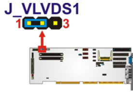
Figure 4-6: LCD Voltage Select Jumper Location
