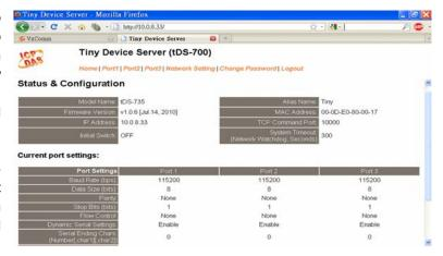
The tDS-700 series also contains a built-in CPU watchdog, which automatically resets the CPU if the built-in firmware is operating abnormally, or if there is no communication between the tDS-700 and the host for a predefined period of time (system timeout). This is an important feature that ensures the tDS-700 operates continuously, even in harsh environments.
