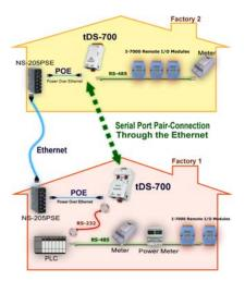
The tDS-700 device servers can be used to create a pair-connection application (as well as serial-bridge or serial-tunnel), and can then route data over TCP/IP between two serial devices, which is useful when connecting mainframe computers, servers or other serial devices that do not themselves have Ethernet capability. By virtue of its protocol independence and flexibility, the tDS-700 meets the demands of virtually any network-enabled application.
