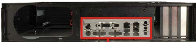
I/O Shield Installed
