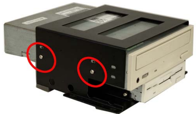
Figure 17: Insert Four Retention Screws into the 5.25" Optical Drive
