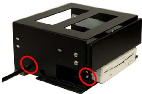
Figure 15: Insert Four Retention Screws into FDD
