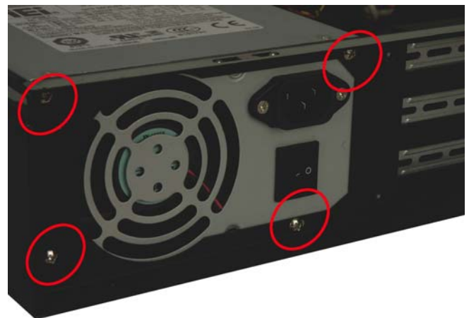
Figure 4: Insert Four PSU Retention Screws
