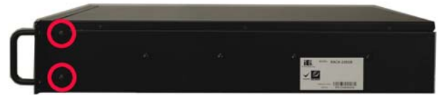
Figure 18: Insert Two Retention Screws for Each Handle
