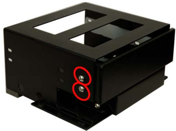
Figure 16: 5.25" Optical Drive Bay Front Cover Retention Screws
