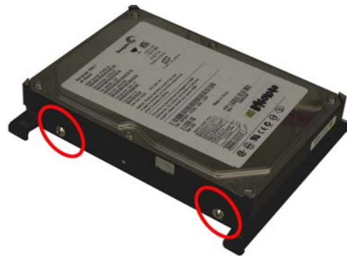
Figure 12: Insert HDD Retention Screws
