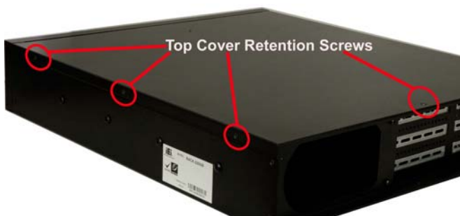
Figure 3: Top Cover Retention Screws
