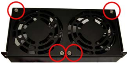
Figure 20: Locations of Fan Retention Screws
