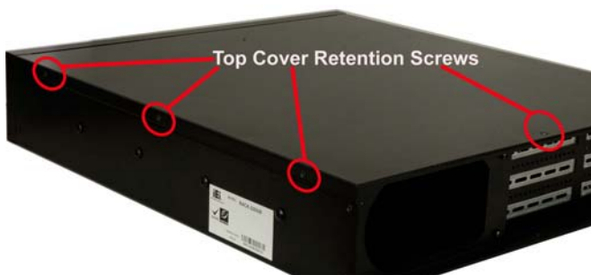
Figure 3: Top Cover Retention Screws
