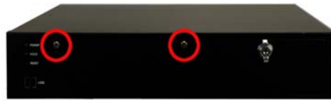
Figure 21: Loosen the Two Thumbscrews on Fan Filter Cover
