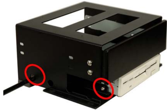
Figure 15: Insert Four Retention Screws into FDD
