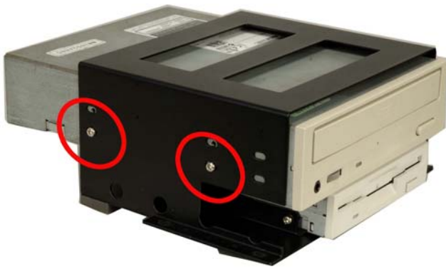
Figure 17: Insert Four Retention Screws into the 5.25" Optical Drive
