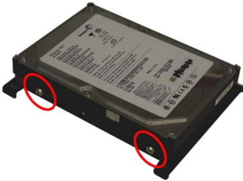
Figure 12: Insert HDD Retention Screws
