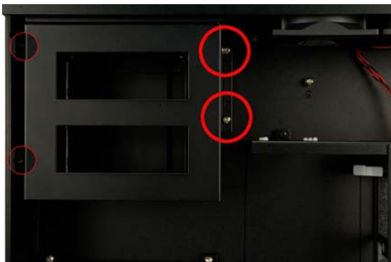
Figure 13: Four Main Drive Bracket Retention Screws
