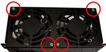
Figure 20: Locations of Fan Retention Screws
