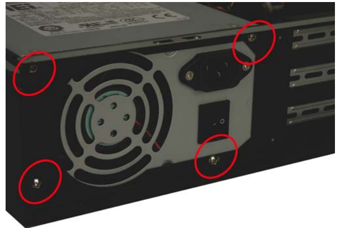
Figure 4: Insert Four PSU Retention Screws
