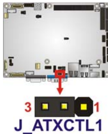
Figure 4-3: AT/ATX Power Select Jumper Location
