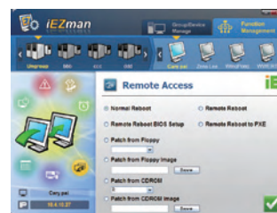
Remote Access Boot the remote PC from a local CD-ROM, floppy drive or ISO image. Or boot into the BIOS
