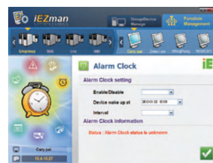
Alarm Clock Sets an alarm to wake the system even under unconnected status
