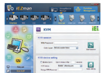
KVM Remote Control (optional) Allow a remote system to control the keyboard, video and mouse with a secure password *VNC license is required
