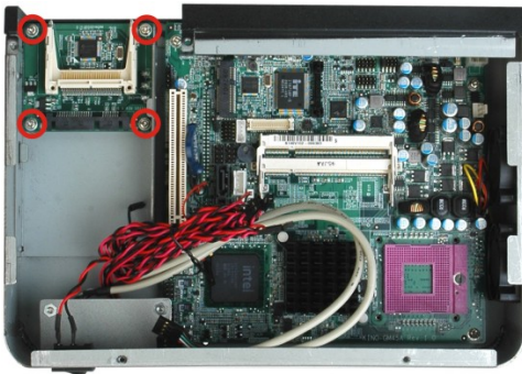
Figure 7: CF Module Installation
