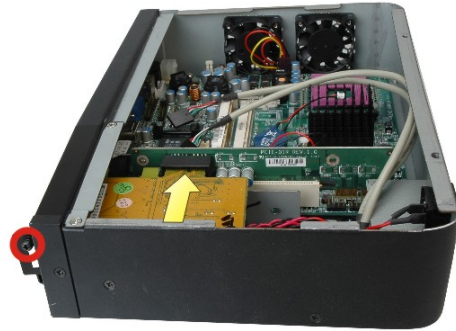
Figure 13: PCI/PCIe Expansion Card Installation
