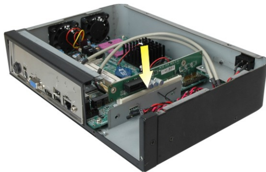
Figure 12: PCI/PCIe Riser Card Installation
