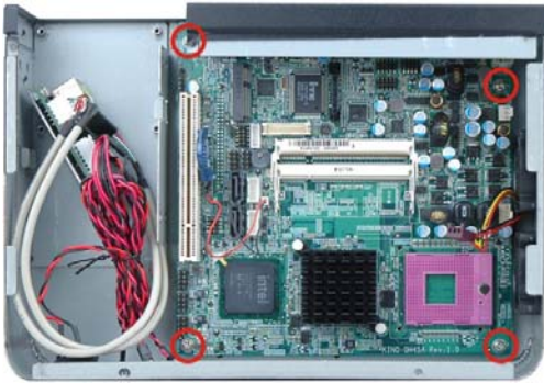
Figure 6: Motherboard Retention Screws
