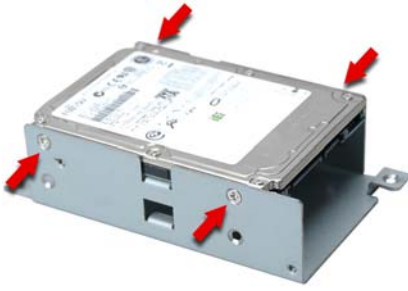
Figure 10: HDD Retention Screws
