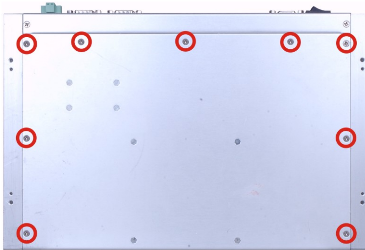
Figure 3-2: Bottom Panel Retention Screws (Bottom Panel)
