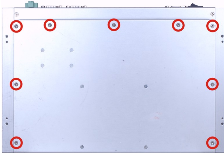
Figure 3-2: Bottom Panel Retention Screws (Bottom Panel)
