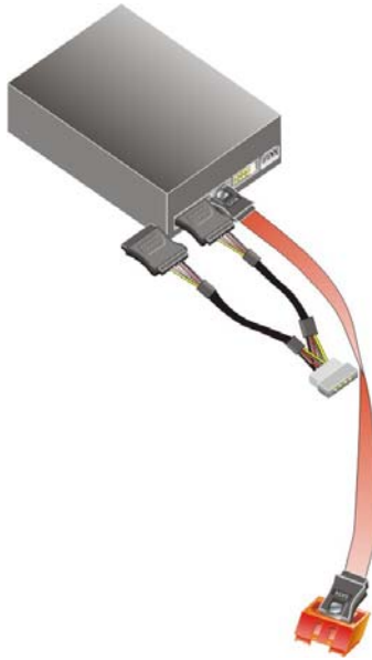
Figure 4-11: SATA Power Drive Connection
