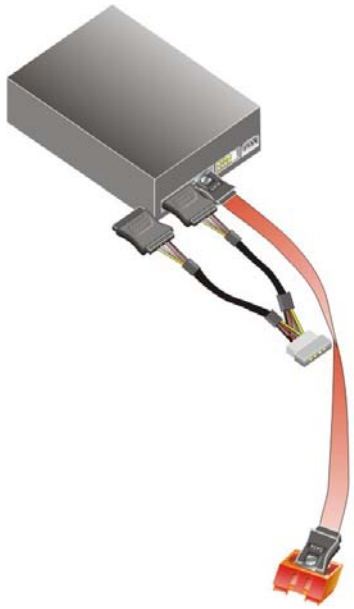
Figure 4-13: SATA Power Drive Connection
