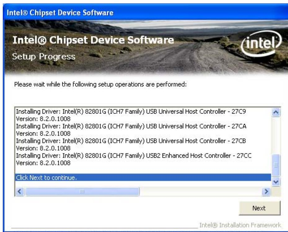
**Figure 6-8: Chipset Driver Setup Operations**
