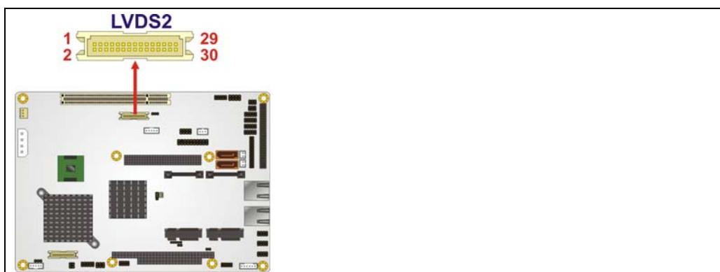
Figure 3-17: LVDS LCD Connector Pinout Location
