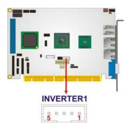
Figure 3-5: LCD Backlight Connector Pinout Locations
