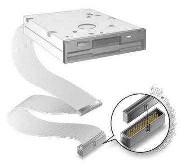
Figure 4-9: FDD Cable Connection
