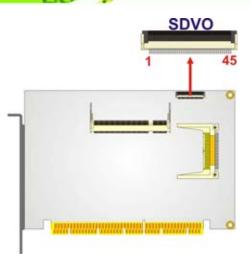
**Figure 3-21: SDVO Connector Pinout Locations**
