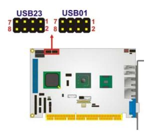
Figure 3-23: USB Connector Pinout Locations
