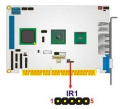
**Figure 3-14: Infrared Connector Pinout Locations**
