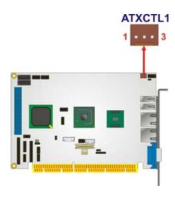
Figure 3-3: ATX Power Supply Enable Connector Location
