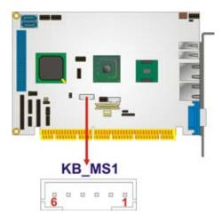
Figure 3-15: Keyboard/Mouse Connector Location
