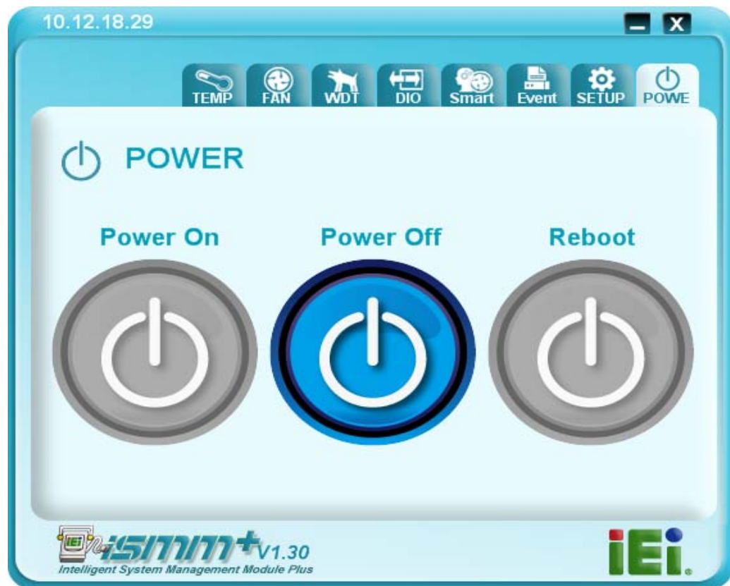
Figure 14: Remote Power On/Power Off /Reboot Page
