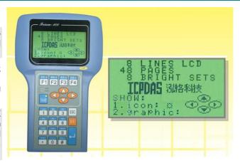
The iVIEW-100 series can be also used as a HMI device for our I-7188, μPAC-7186 and I-8000 series embedded controller. Since the basic hardware design of iVIEW-100 is similar to that of I-7188 series, all our available software can be used in iVIEW-100. User can design iVIEW-100 application with C Language. We will provide iVIEW-100E with a 10/100 mega Ethernet port for internet.
