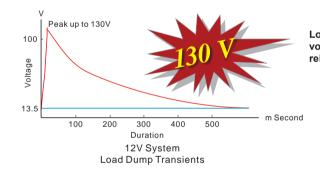
Load dump transients typically reach peak voltages of 130 volts in 12 volt systems with relatively slow rise times.
