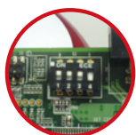
The ID is programmed by a 4-digit DIP switch
