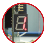
Digit LED to show its ID (identification)
