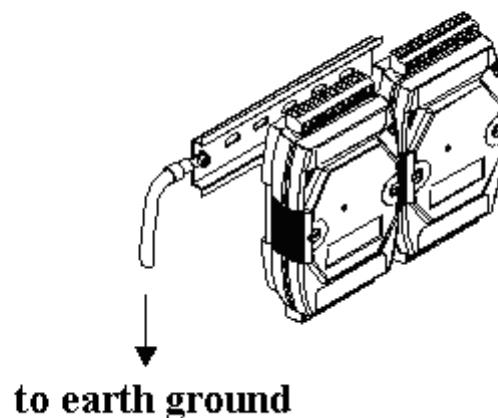
**Note:** The recommended wire to connect to the earth ground is 16 – 14 AWG wire.
